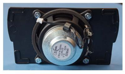
The back of the plate has four corner bosses that hold the assembly firmly in the case slot. The speaker & plate assembly must fit snugly in the slot once the two case halves are assembled.
